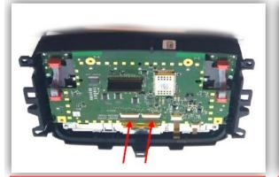
**Step5:** Disconnect the 2 LCD ribbon cables from main board carefully.
