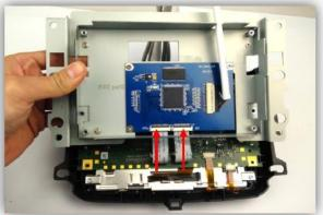
**Step8:** Connect OE Golden Ribbon cables back to Daughter PCB Board to complete the connection.
