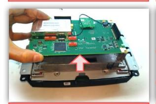
**Step3:** Carefully remove the PCB board as shown.
