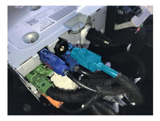
Insert the blue image connector of the interface Y-cable in the headunit, and insert the OEM LVDS cable in the female connector left side (install in between)
