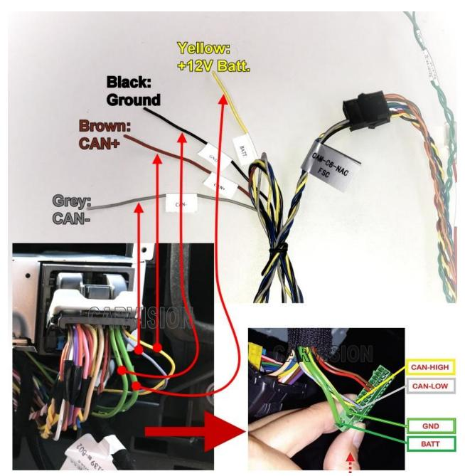
Connect power and CAN as below. Check power signals of the headunit first to avoid short circuits
