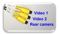
We recommend to **power the rear camera by using the RED(12V) + BLACK(GND) wires of the interface** instead of backlights to avoid distortion in camera image, especially when the engine is running!
