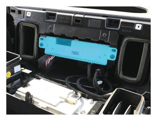
Take out the OEM <u>black</u> LVDS cable from the headunit. The position of this cable can be different.
