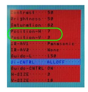
The UI-CONTROL option: set the PDC picture display on/off . It's another function is to toggle the Chinese Caption ON/OFF on screen.
