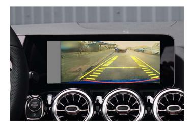
Adjust "position H" (horizontal) to move the image to the left ← or right →
