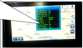
The "Guide CTRL.....ON": the installer can set ON/OFF to enable the parking guide line, which shows the safe zone when parking. please set to OFF.
